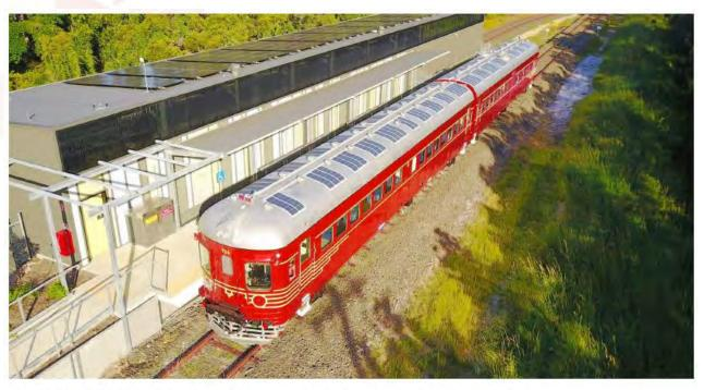
Australia | SMF35M-2x6UW | Gluing via silicone sealant for PV modules The world's first solar-powered train, blending heritage with modern technology.
