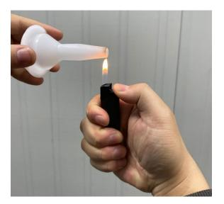
2. It is recommended to use a lighter to heat the tip of the rubber nozzle for about 2s to prevent it from springing back after being flattened.
