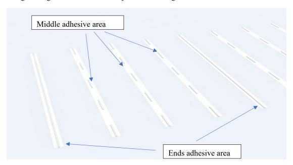
■ Paste the rail along the gluing path, lightly compress, keep the glue thickness is not less than 3mm
