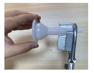
1. Use a straightedge or tape measure to measure the length of the head of the nozzle 20mm, confirm the cutting position, and then use the tool to cut in addition.
