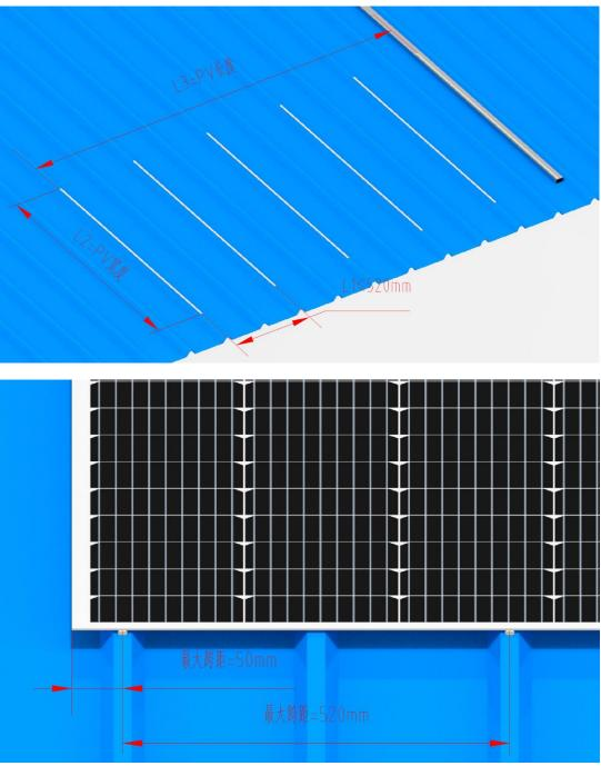
■ If there is a joint in the aluminum tube, the priority is to put the joint between the modules.
