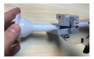
3. Squeezing of the nozzle to the desired size using a flattening die of the tool shears.
