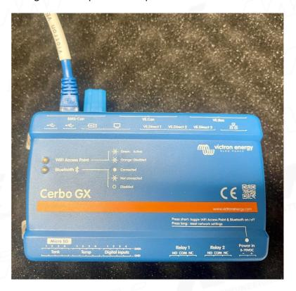
2. Type A Victron Can-Bus cable directly into the GX devices VE-CAN port (Cerbo-S). Example:
